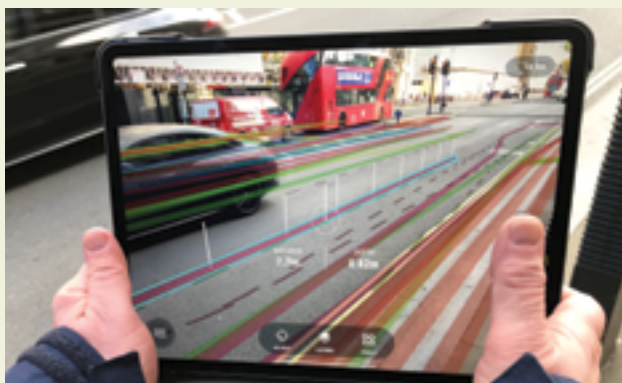
Examples of images generated by software – highlighting services location
