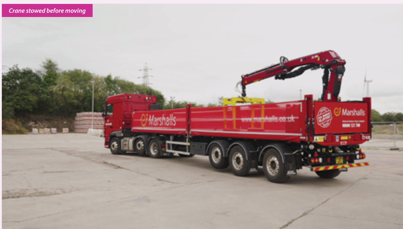
Driver cannot remove keys until crane lowered
